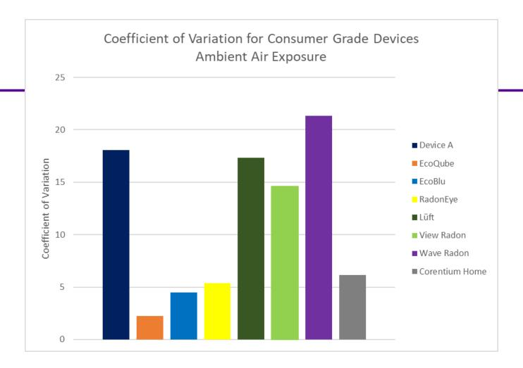
Coefficient of Variation (CV): The ratio of the standard deviation to the mean. The higher the CV, the greater dispersion around the mean.
