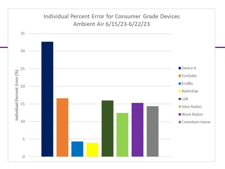
Individual Percent Error (IPE): The degree from which a single measure value (X) deviates from the conventionally true value (T)
