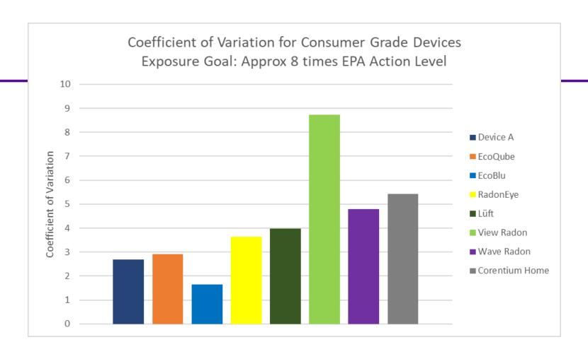
Coefficient of Variation (CV): The ratio of the standard deviation to the mean. The higher the CV, the greater dispersion around the mean.
