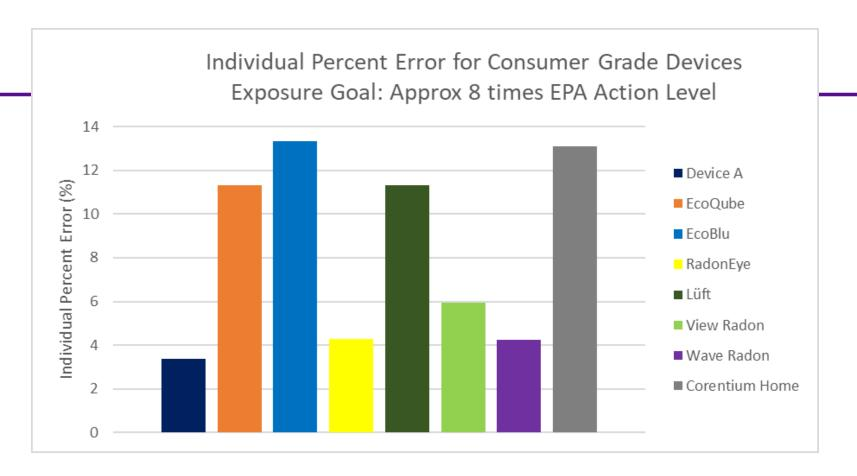
Individual Percent Error (IPE): The degree from which a single measure value (X) deviates from the conventionally true value (T)
