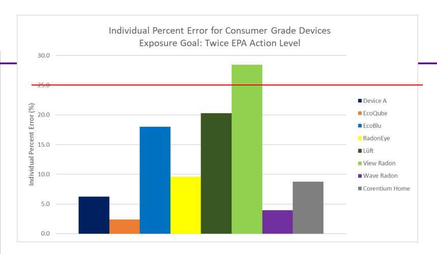
Individual Percent Error (IPE): The degree from which a single measure value (X) deviates from the conventionally true value (T)
