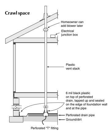
Crawlspace with passive radon-resistant technique
