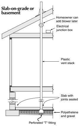
Slab foundation with passive radon-resistant technique
